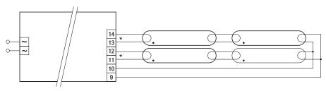
\* leads 11, 12, 13, 14 max. 1.0 m (< 100 pF) leads 9, 10 max. 2.0 m (< 200 pF) Protection class I – luminaires: earth of ballast housing required (according to IEC 598) Protection class II – luminaires: no earth required
