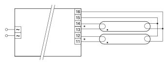
leads 11, 12, 13, 14 max. 1,0 m (< 100 pF) leads 15, 16 max. 2,0 m (< 200 pF) Protection class I – luminaires: earth of ballast housing required (according to IEC 598) Protection class II – luminaires: no earth required
